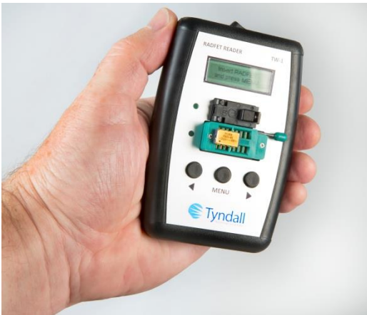
Handheld RADFET reader developed at Tyndall.
